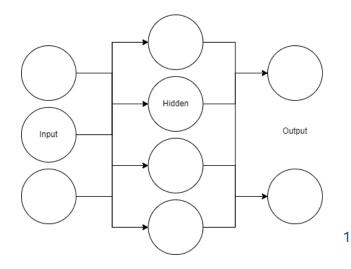
The input layer receives the raw data (This can be image, audio, video, text etc.) each neuron in the input layer corresponds to a feature of the data (Example 1, Image 28x28 = 784 pixels, therefore 784 neurons, each neuron receives a pixel. Example 2, Large text file, split into vectors, each neuron receives a vector.) it will then pass it on.
